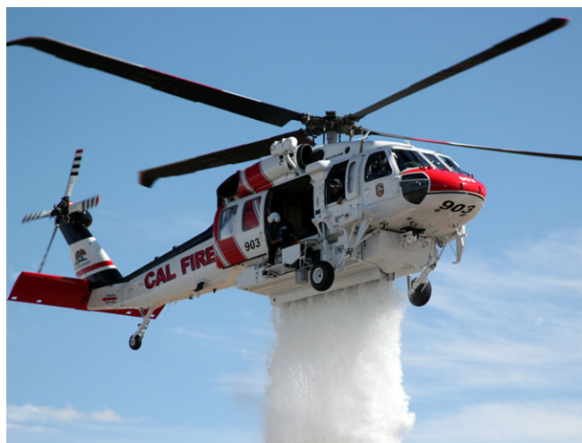
Figure 4. External hard-sided tank on a FIREHAWK ® . 7
