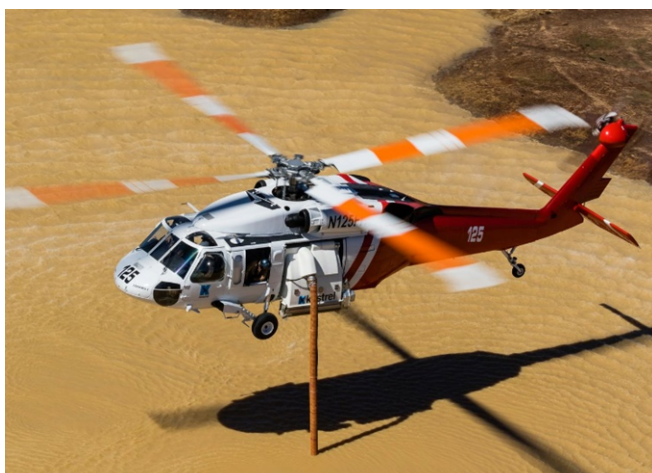
Figure 3. Internal water tank with snorkel. 6
