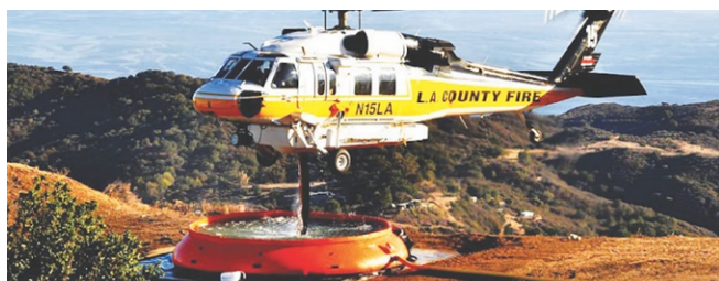
Figure 7. L.A. County FIREHAWK® filling from a remote fill tank at 69 Bravo Helistop. 11,12
